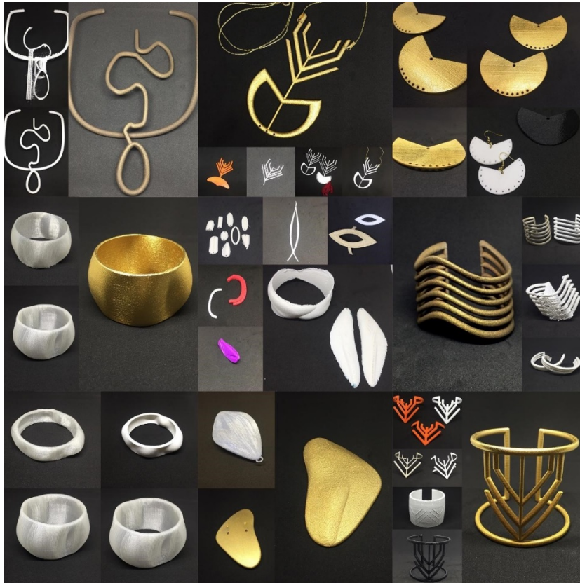
Figure 3. The application of 3DP to this design process allowed for rapid prototyping/evaluation/and refinement in a circular loop. Pictured here are various prototypes at multiple stages of development in materials including PLA, plastic, and steel.
